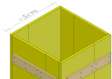
In order to close the edges of the column, one pair of panels should have the same width as the pillar, the other pair have to be 5 cm wider
