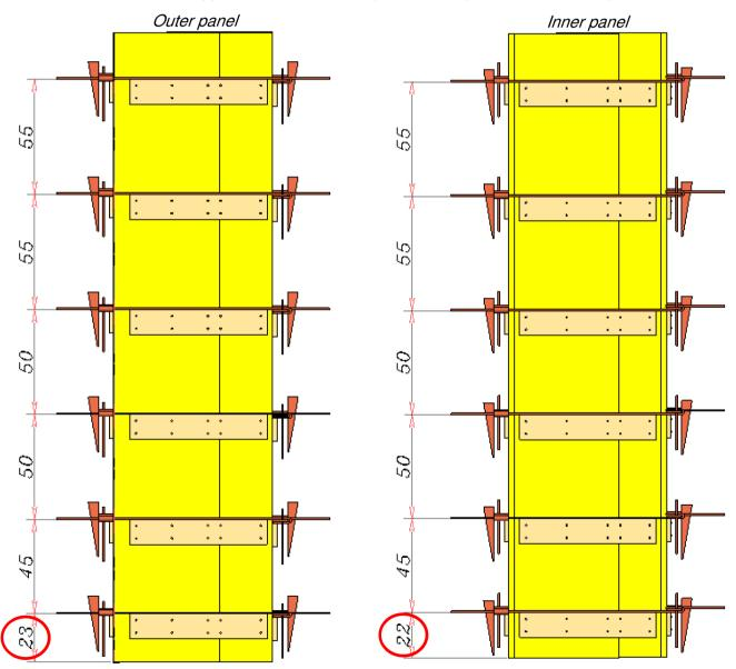
The boards of the outer panels have to be 1 cm higher than the boards of the inner panels
