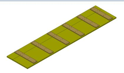
The boards will be used as a support for the ties, so they have to be positioned with the proper wheelbase
